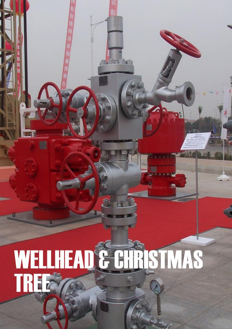
Wellhead And Christmas Tree Equipment can be mainly used in Continental flowing wells, pumping wells, pump wells, screw pump oil wells.
